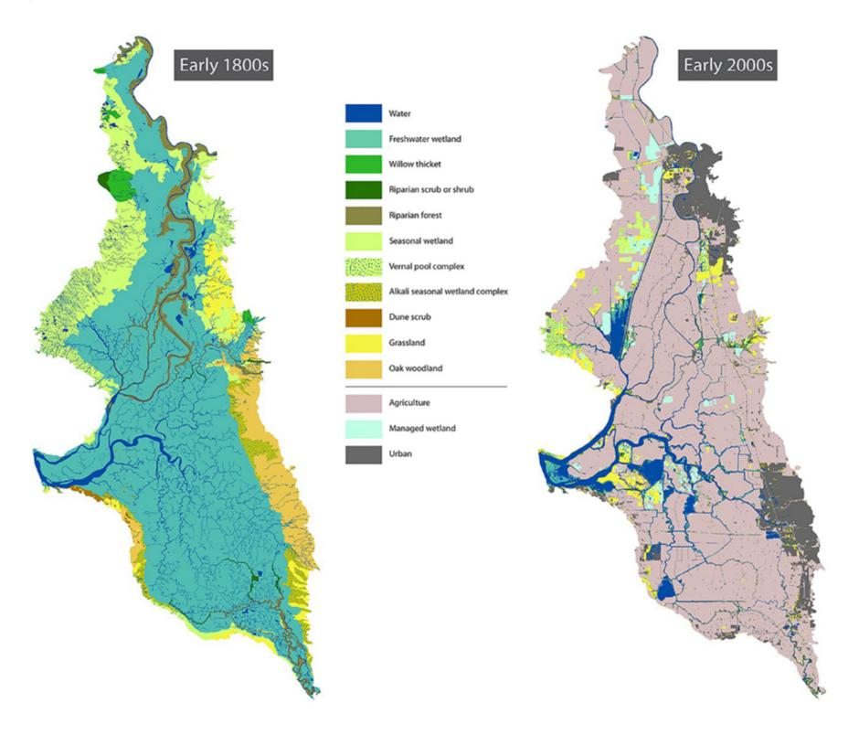
FIGURE 3. Maps of the Delta showing the transformation from a complex system of river and distributary channels of multiple sizes and shapes to the present water transport system dominated by straightened and simplified channels. Transformation also included a major simplification of native landscape types to an agriculturally dominated landscape. From the Sacramento-San Joaquin Delta Historical Ecology Study, available at: www.sfei.org/DeltaHEStudy (Whipple et al. 2012)
